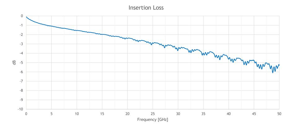
De-Embedded physical measurements of micro-LinkOVER Assembly (micro-LinkOVER to micro-LinkOVER) with 8" of 95
