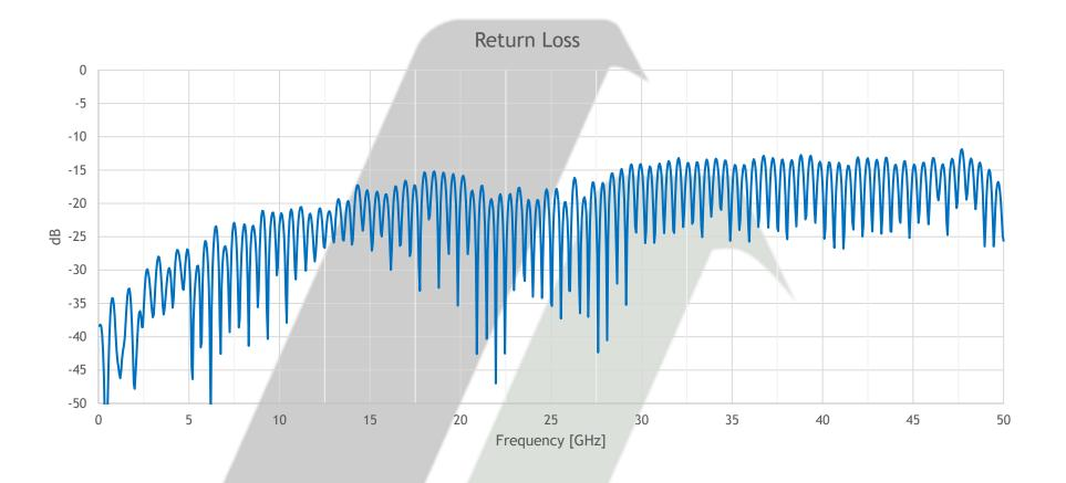
De-Embedded physical measurements of micro-LinkOVER Assembly (micro-LinkOVER to micro-LinkOVER) with 8" of 95 Ω 32 AWG cable. Measured data of the micro-LinkOVER with a stripline differential trace length of 2 mm made with Tachyon Dk 3.25 10 mils thick.
