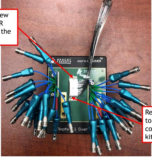
Remove M1.6 Pan Head Screw to separate micro-LinkOVER connector from the rest of the kit
