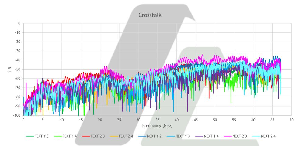
NEXT and FEXT with two TR70-03VF fixtures of μLO to μLO with eight inches of 95 Ω 32 AWG twinax cable on GCPW Stripline Differential with Tachyon Dk 3.25 10 mils thick.
